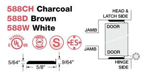
1/8" clearance required between door and frame
