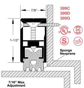
**PLEASE NOTE:** These products have been fire rated for use as perimeter seals only and shall not be used in lieu of an integral pressed steel stop on fire rated installations.
