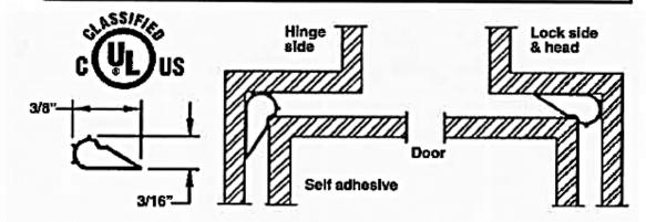
Category J Gaskets for use with Listed steel frames and/or Classified steel covered composite, hollow metal doors rated up to 3 hrs; wood and plastic covered composite doors rated up to 1-1/2 hrs and wood core doors rated for 20 minutes. Meets CAN4-S104-2010.
